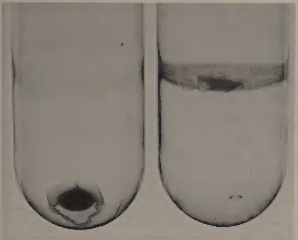
Figure 6. Competency of cardiac SR vesicles. Cardiac SR vesicles were loaded in the presence (left) or absence (right) of oxalate, layered over 40% sucrose, and then centrifuged. Calcium oxalate-loaded vesicles penetrated the 40% sucrose and were collected as a pellet. A small proportion (about 14%) of material failed to load with calcium oxalate.
